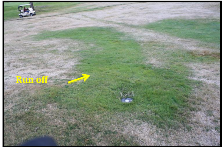
Sunken head deflects spray causing water run off
